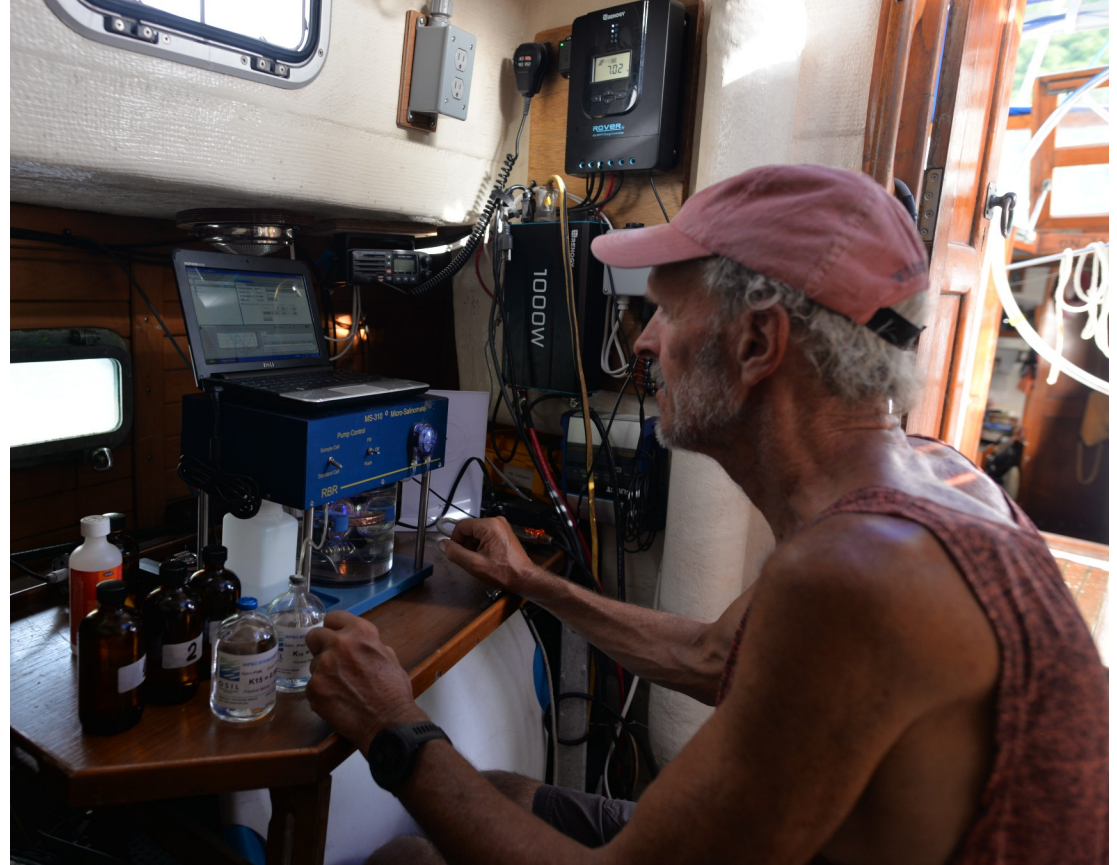
Operating Micro-Salinometer in Oceanographic lab onboard SV Oceanolog. T=32degC, no an air conditioner needs!
